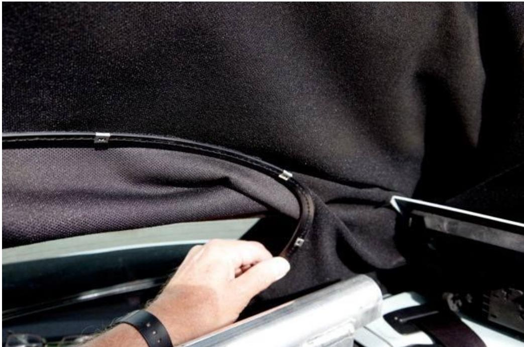
With the clips installed fold the headliner edge beading over (flip it) into the metal retaining channel around the glass.
