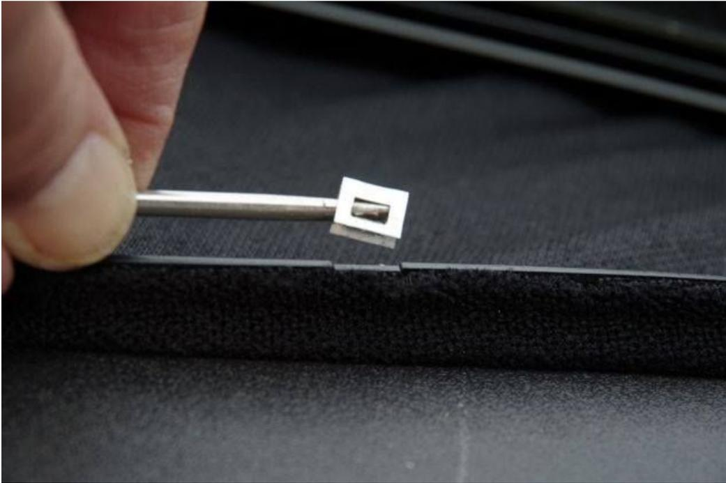
Install 18 clips around the headliner beading, one at each notch (see above image) cut into the beading as shown in the image below.
