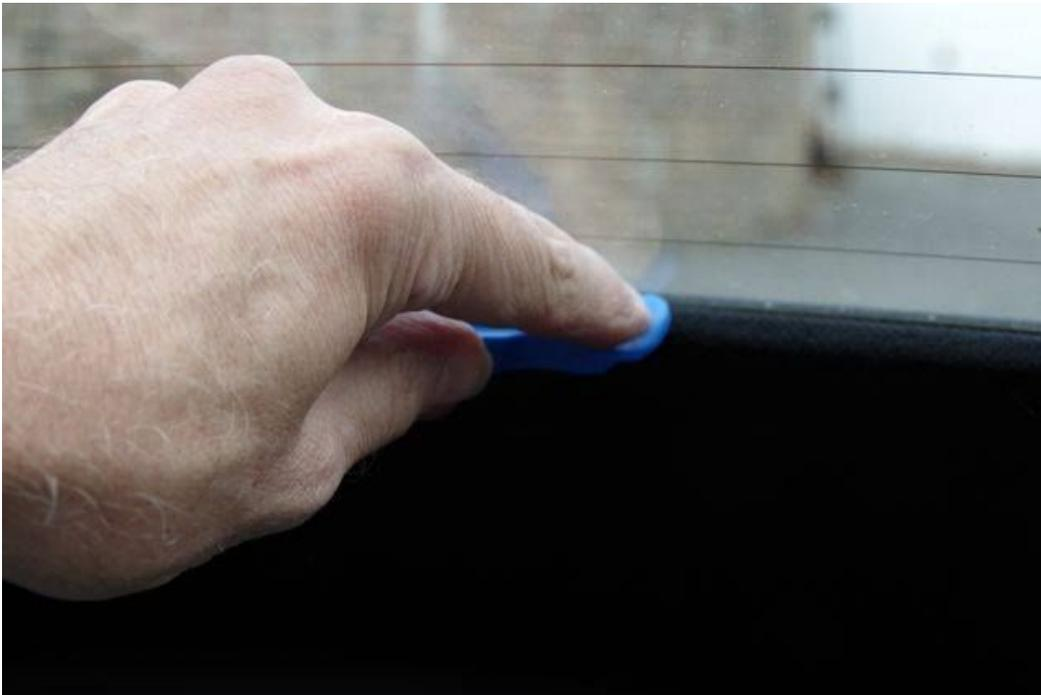
If necessary use a wide smooth edged nylon block or flat wooden implement and a rubber/plastic mallet against the cloth of the headliner (**do not damage the headliner**). Tap lightly all around the channel until the beading is evenly seated.
