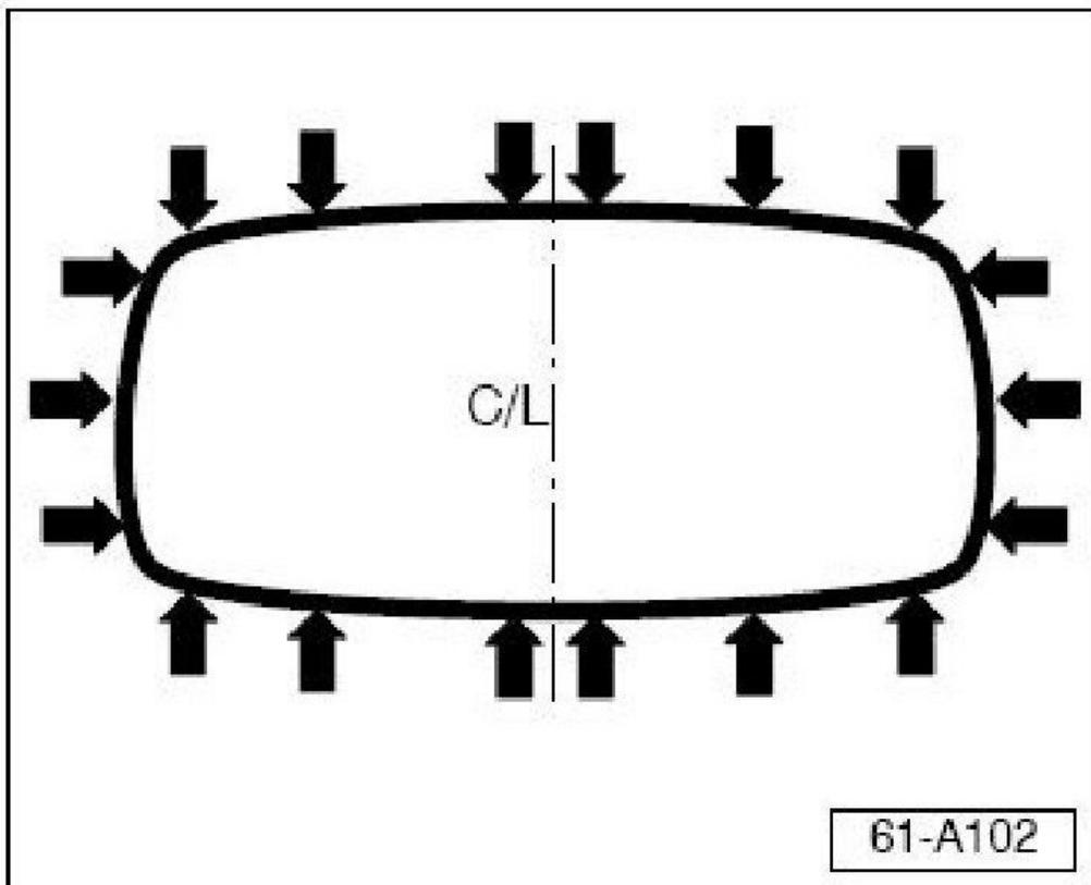
\*Clips must be installed using flat pliers (plastic or with jaws protected) at the plastic beading edge. Clips must go over the plastic beading only (**headliner cloth must not interfere**).
