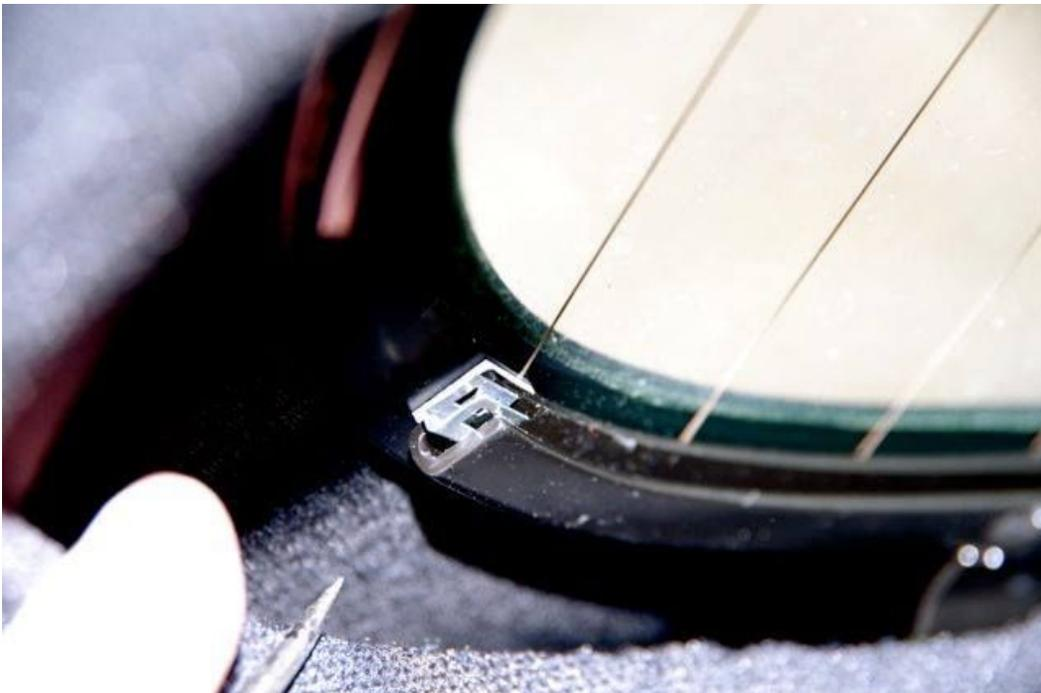
\*Check for any dislodged black plastic/silver metal insert clips and remove them from the black metal channel.
