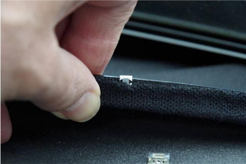
It may be necessary to gently press the beading into the retainer.
